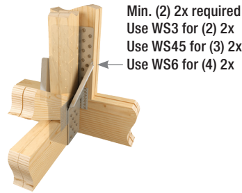
Typical GTQ218 installation (GTQM218 similar)
